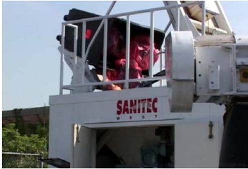
**FIGURE 2.** An automatic lift-and-load system protects workers from devastating back injuries.
